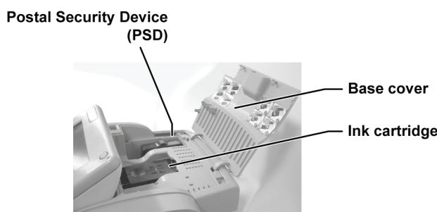
Figure 2 : Base internal details
