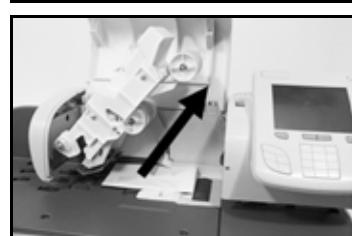
6 Push down on the upper drive assembly until it locks back into position.
