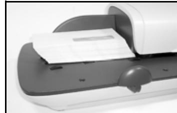
Ensure that all the envelopes are stacked along the rear guide, from largest to smallest.
